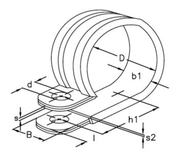
$\begin{array}{lll} b1 & = 12.5 \\ d & = 4.3 \\ Diameter D = 20 \\ h1 & = 15.7 \\ I & = 3.8 \\ s & = 0.40 \\ s2 & = 1.0 \\ Width B & = 9 \end{array}$
